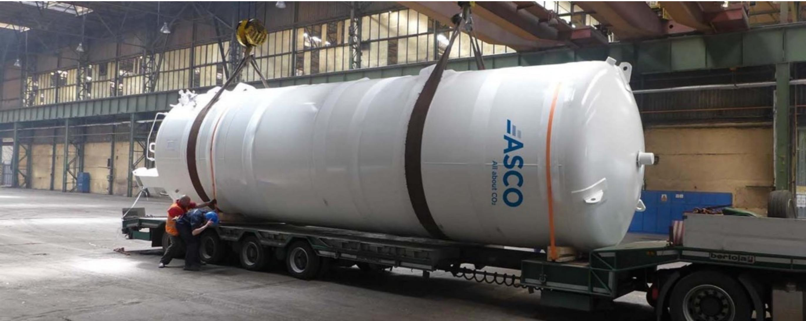
**Typical 30 ton Tank for storage liquid CO<sub>2</sub>**
