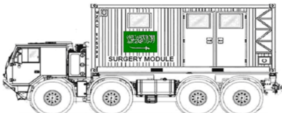
T 815 OFF ROAD TRUCK 8 x 8 WITH SURGICAL CONTAINER ISO 1 CC (20 FEET)
