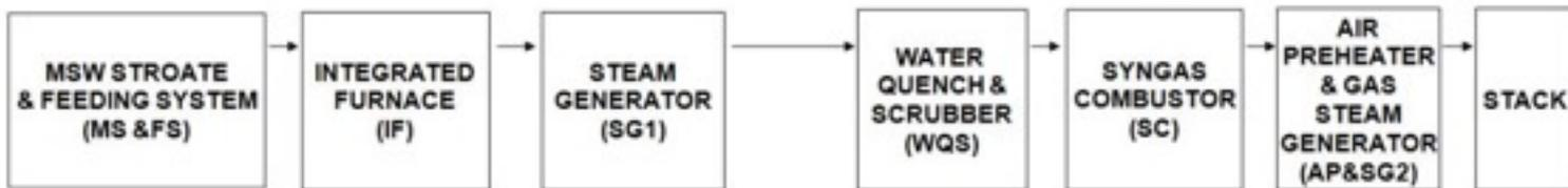
**Plasma Gasification is an extreme Thermal Process using Plasma which converts Organic Matter into a Syngas (Synthesis Gas) which is primarily made up of Hydrogen and Carbon Monoxide.**
